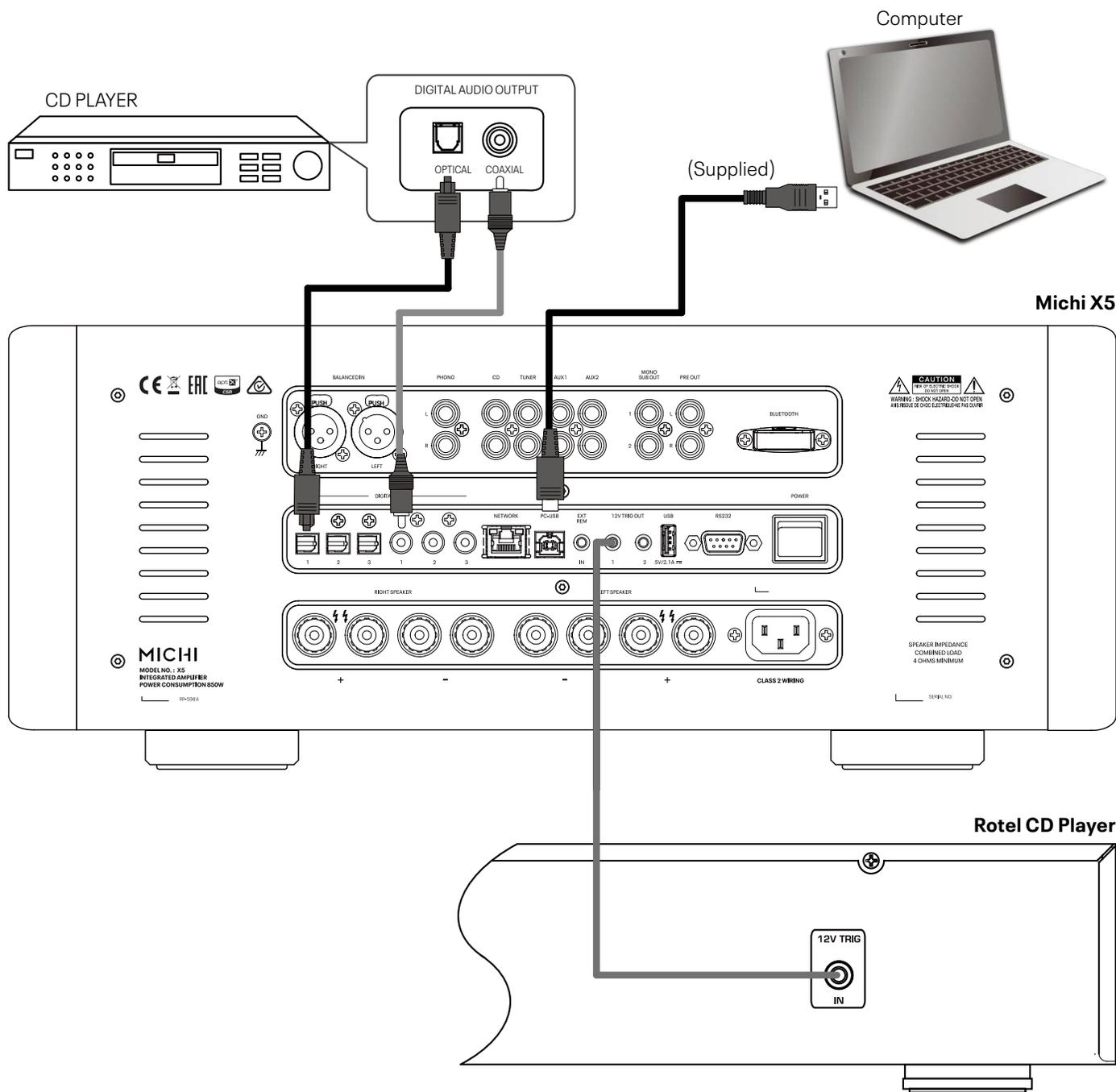
**Figure 5: Balanced (XLR) Inputs**
