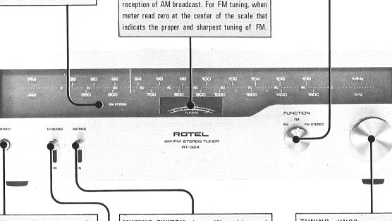
POWER SWITCH: supplies power to the tuner. When the switch is ON, dial scale will he illuminated.
