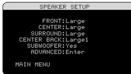
The SPEAKER SETUP menu is used to configure the RSX-1058 for use with your specific loudspeakers and to determine the bass management configuration as described in the previous overview. The menu is accessed from the MAIN menu.
