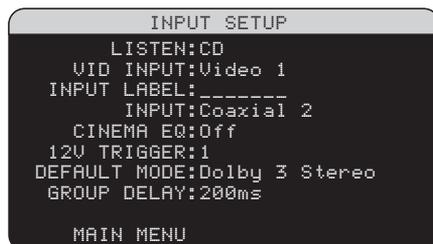
The INPUT SETUP menu configures the source inputs and is reached from the MAIN menu. The screen provides the following options, selected by placing the highlight on the desired line using the UP/DOWN buttons:
