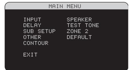
The MAIN MENU provides access to OSD screens for various configuration options. MAIN MENU is reached by pressing the ENTER button from the SYSTEM STATUS menu described above or from most other menus. To go to the desired menu, move the highlight using the UP/DOWN and +/- buttons on the remote and press the ENTER button. Press the MENU/OSD button on the remote to cancel the display and return to normal operation.
