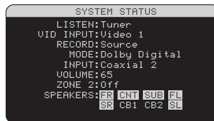
The SYSTEM STATUS menu provides a snapshot of the current system settings and a starting point for reaching all other screens and menus. This screen appears when you press the remote MENU/OSD and displays the following information:
