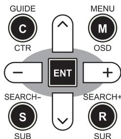
**MENU/OSD button:** Press to display the SYSTEM STATUS screen. From the SYSTEM STATUS screen, press the ENTER button to display the MAIN MENU screen which has links to all other menus. If a menu is already
