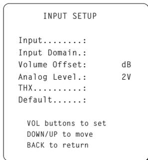
The RSP-985 accepts both analog and digital signals. The INPUT SETUP menu allows you to configure each input:
