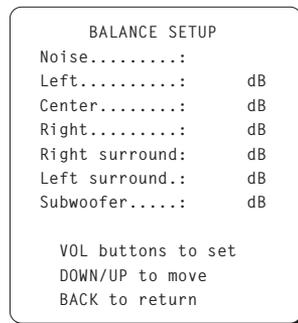
This menu, also reached from the MAIN screen, adjusts the relative volume level of all six speakers. Just as you set the delays in the previous step to ensure that the sound from all of the speakers arrives at the same time, you also need to ensure that the volume of the sound from all speakers is the same.
