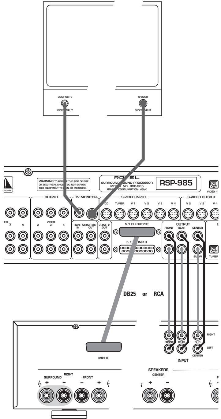
Figure 4 – RCA Source Connections
