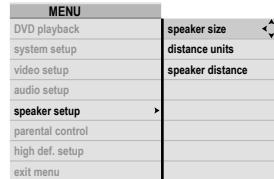
The Speaker Setup menu provides three setup items relating to surround sound and bass management of the audio signals at the analog outputs of the RDV-1093.
