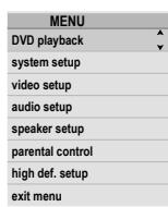
2. Press the CURSOR ▲/▼ buttons to highlight the desired item and press the ENTER button or the CURSOR ► button to display the corresponding pop-up Options Menu. In this example, the options for the DVD playback selection are shown:
