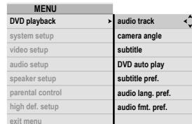
There are seven items on the DVD playback options menu when a disc is inserted in the RDV-1093. If a disc is not inserted the four options under the DVD auto play item are shown automatically.
