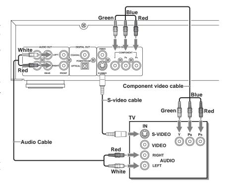
**NOTE:** See the Video Signal Selector Switches section for information on setting the switch for the various types of connections.
