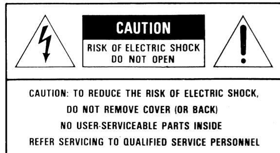
The lighting flash with arrowhead symbol, within an equilateral triangle, is intended to alert the user to the presence of uninsulated "dangerous voltage" within the product's enclosure that may be of sufficient magnitude to constitute a risk of electric shock to persons.
