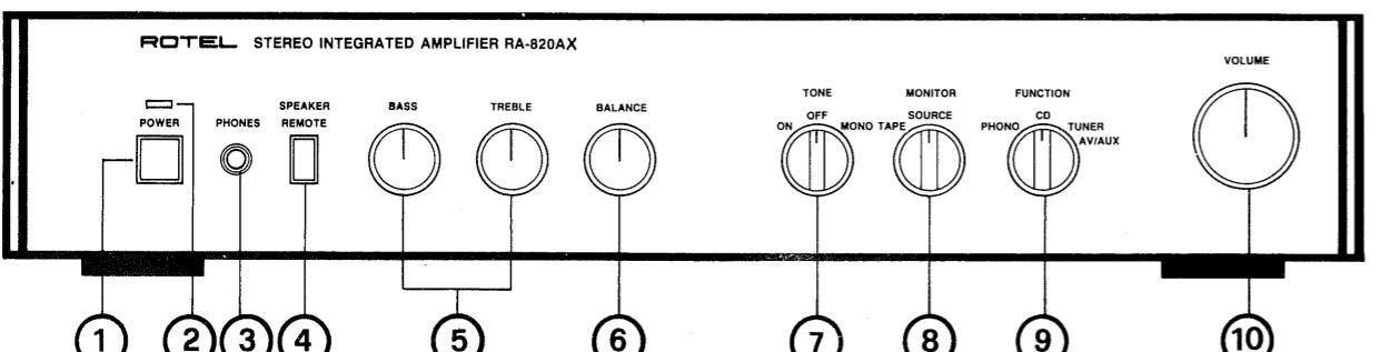
When the SPEAKER REMOTE button is at OFF, the sound from the speakers connected to the REMOTE SPEAKERS terminals is cut off and you can adjust the headphone volume with the VOLUME control.
