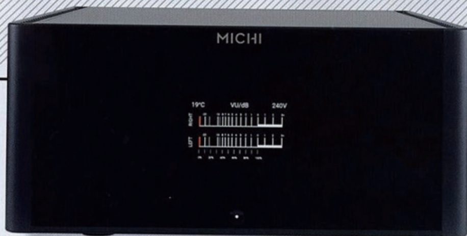
ABOVE: Front panel of the S5 power amplifier is as understated as that of the preamp – well, except for the prominent display, which can be switched between VU meters and a choice of 'Frequency Spectrum Analyser' readouts, with 8, 12 or 16 bands. Fortunately, it can also be turned off...
