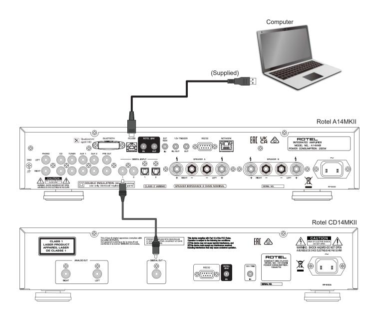
Figure 5: 12V Trigger Connection
