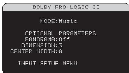
When Dolby Pro Logic II is selected as the default surround mode on the INPUT SETUP menu, there are additional settings and parameters to optimize the surround decoding for music or movie soundtracks. Dolby Pro Logic II uses matrix decoding algorithms to derive a center channel and surround channels from 2-channel source material.
