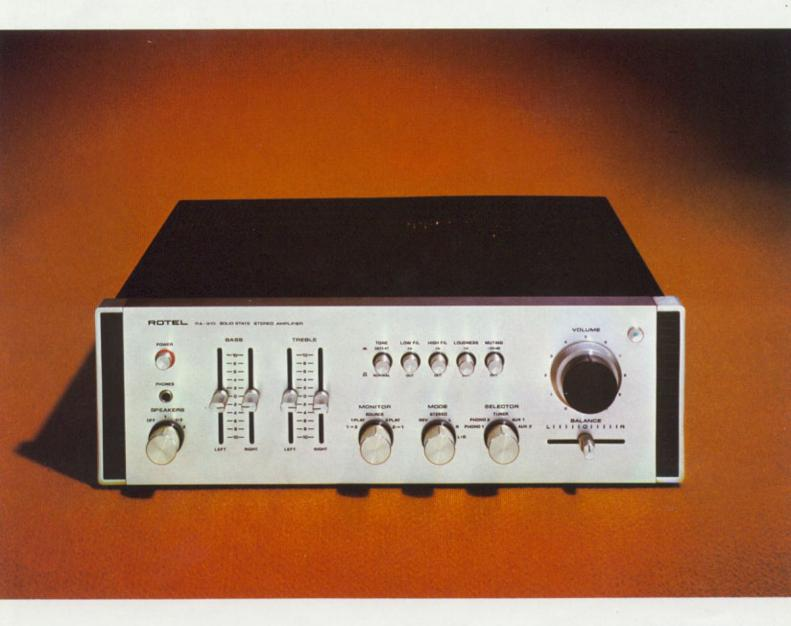
HERE is the RA-810 propably one of the most versatile, most professional stereo pre-main amplifiers ever developed. Possessing an abundant 180 watts music power, the specially designed split power supply drives almost any quality speakers stably and smoothly. The direct coupling circuitry incorporated ensures an excellent frequency response and negligible IM distortion. The transistors used are
