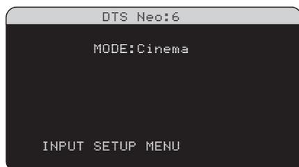
When DTS Neo:6 is selected as the default surround mode on the INPUT SETUP menu, there are additional option settings and parameters available to optimize the surround decoding for various types of recordings, music or movie soundtracks. DTS Neo:6 uses matrix decoding algorithms to derive a center channel and surround channels from 2-channel source material.
