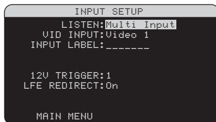
When the MULTI INPUT source is selected on the INPUT SETUP menu, the available options change to reflect the fact that these inputs are direct analog inputs and bypass the RSX-1057's digital processing. The INPUT, CINEMA EQ, and DEFAULT MODE options are not available since these are all digitally implemented features.
