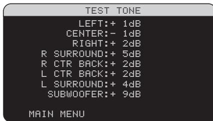
This menu uses filtered pink noise test tones to set equal volume levels for all speakers (left front, center, right front, right surround, center back, left surround, and subwoofer) to ensure proper surround sound reproduction. Setting the output levels using the test procedure provides the most accurate adjustment so that digital surround sound material will be reproduced as it was intended and is a critical step in calibrating the system.
