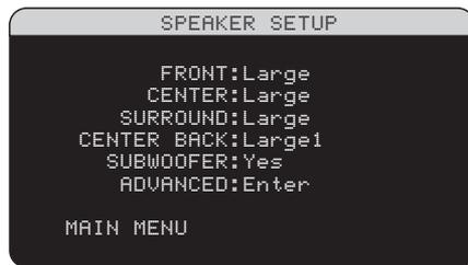
The SPEAKER SETUP menu is used to configure the RSX-1057 for use with your specific loudspeakers and to determine the bass management configuration as described in the previous overview. The menu is accessed from the MAIN menu.
